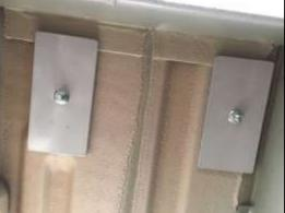
Screw the provided 3/8-16 hex head lock nuts on to the mounting bolts and tighten until the console and waste tank are firmly attached to the vehicle floor.
