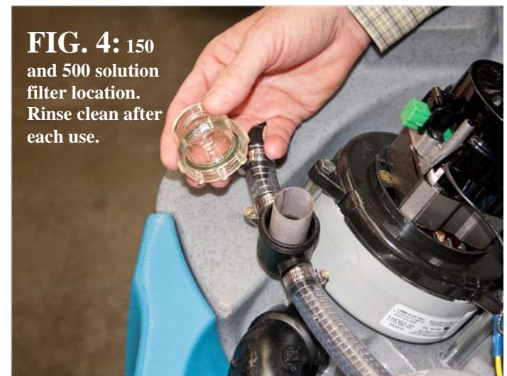
**FIG. 4: 150 and 500 solution filter location.
