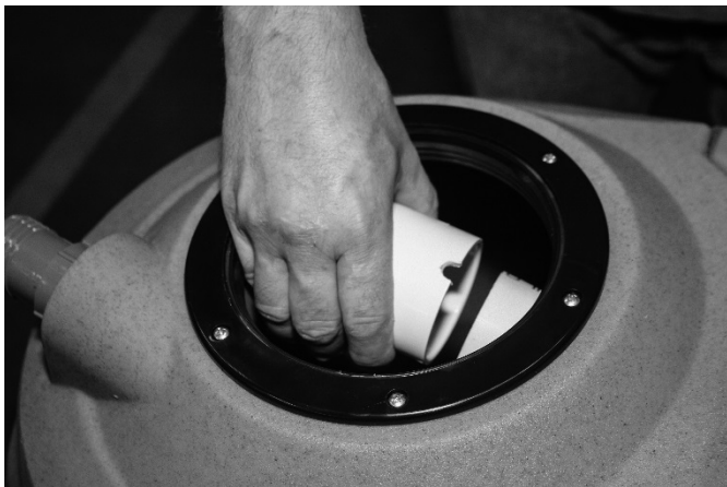
FIG. 5: Vacuum cutoff valve removal and cleaning
