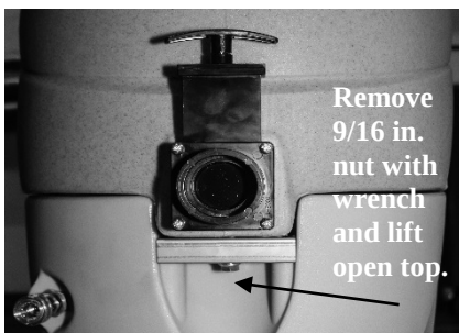
FIG. 4: Solution inlet filter cleaning
