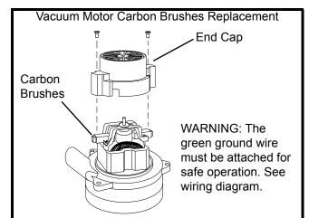
If armature commutator is grooved, extremely pitted or not concentric, the motor will need to be replaced or sent to a qualified service center.
