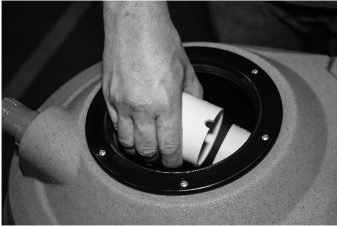
FIG. 5: Vacuum cutoff valve removal and cleaning
