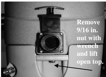
FIG. 4: Solution inlet filter cleaning
