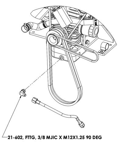
The part number for the Legend Brands 570 Truckmount engine oil drain fitting, 21-142, has been obsoleted for ALL serial number ranges of the 570 Truckmount. This fitting has been replaced with Legend Brands part number 21-602. This has always been a proprietary part and cannot be replaced with an off-the-shelf component. Please contact Legend Brands for 21-602 when ordering a replacement oil drain fitting for ANY 570 Truckmount unit.
