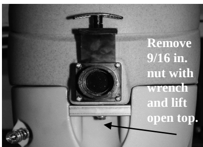
FIG. 4: Solution inlet filter cleaning
