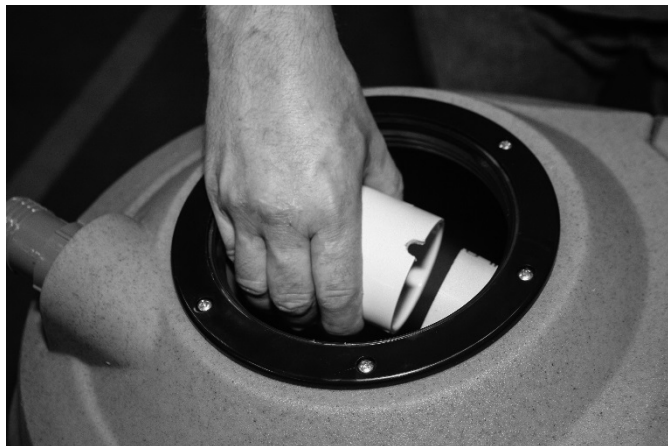
FIG. 5: Vacuum cutoff valve removal and cleaning
