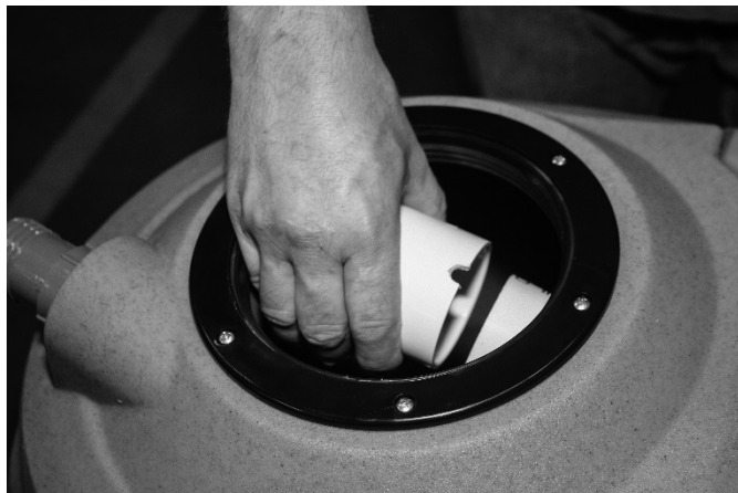
FIG. 5: Vacuum cutoff valve removal and cleaning
