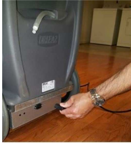
CORRECT PLUG REMOVAL Models F410 & F411 Grasp IEC plug and pull straight out
