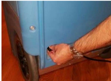
INCORRECT PLUG REMOVAL Models F410 & F411 Models F412 & F532
